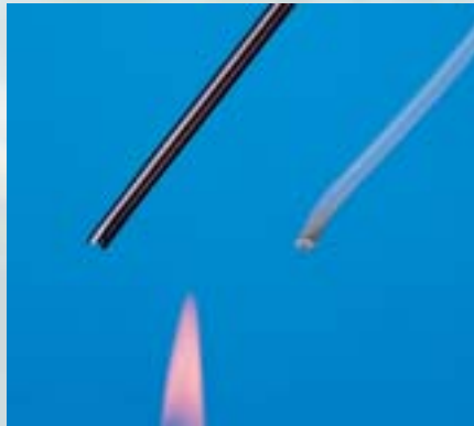
FEP tubing softening after one minute in contact with 300°C flame.
