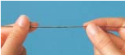
Upper FEP tubing is less rigid, even harder to pass a conductor through.
