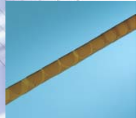
Spiral tubing loosening in contact with 300°C flame.
